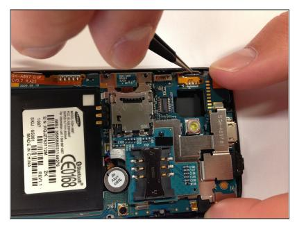
• Use the tweezers to unclip the other orange ribbon cable along the left side of the phone.
