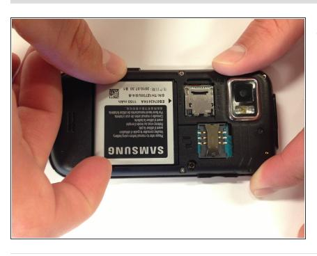
Place your finger on either bottom corner of the battery slot and lift to remove the battery.
