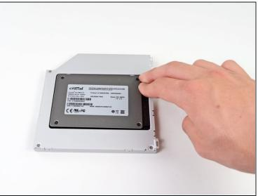
Once the hard drive is snug, reinsert the plastic spacer while holding the hard drive against the bottom of the enclosure.
