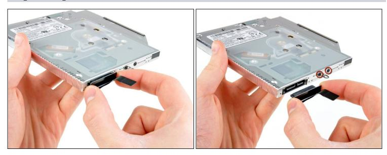
• Pull the optical drive cable away from the optical drive.
