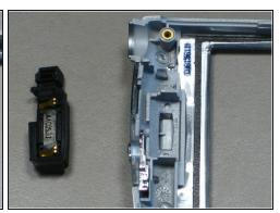
• Pull out the earphone by grabbing the black rubber piece identified in the picture.
