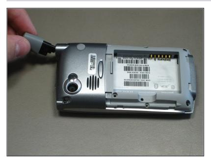
Pull the antenna outward to remove the antenna from the body of the phone.
