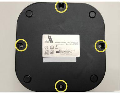
The device can be opened by removing the 4 Philips screws visible from the bottom
