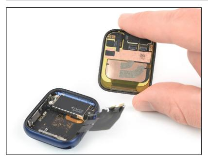
Separate the watch assembly and the screen.
