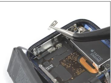
• Use a pair of tweezers to remove the metal shield covering the battery connector.
