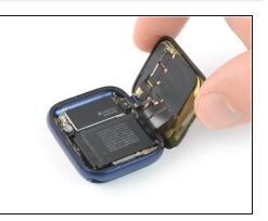
⚠ Be careful not to strain the display cables when you fold the display to the side.
