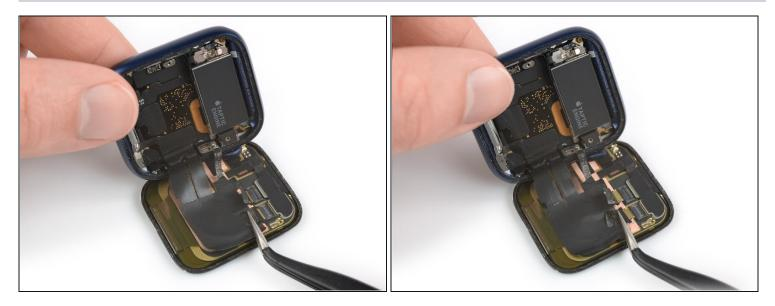
Use a pair of tweezers to pull both display cables out of the ZIF connectors.
