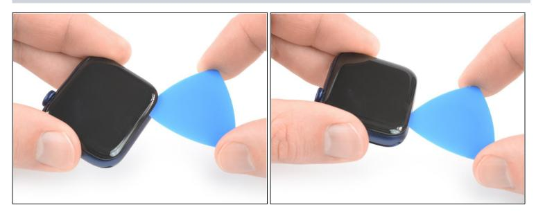
Slide the opening pick around the corner and along the long edge on the opposite side of the watch crown to cut the display adhesive.
