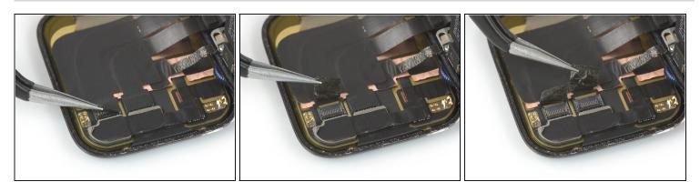
Use a pair of tweezers to carefully peel the black protective tape off both display connectors.
