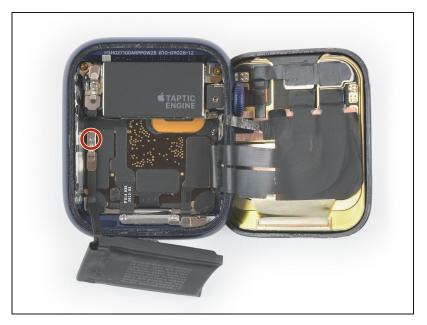
Remove the single 1.2 mm-long tri point Y000 screw.
