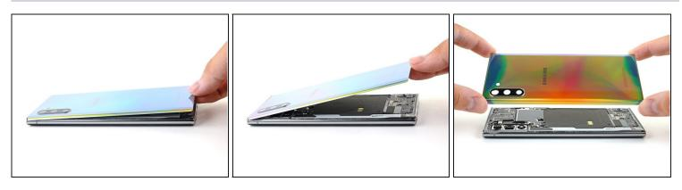
Lift up and remove the back panel.
