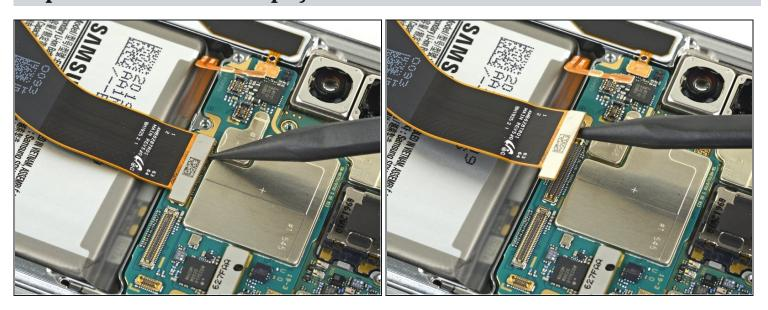
• Use the pointed end of a spudger to disconnect the display cable connector from the motherboard.
