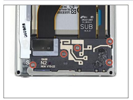
Use a Phillips screwdriver to remove the five 4 mm screws securing the loudspeaker.
