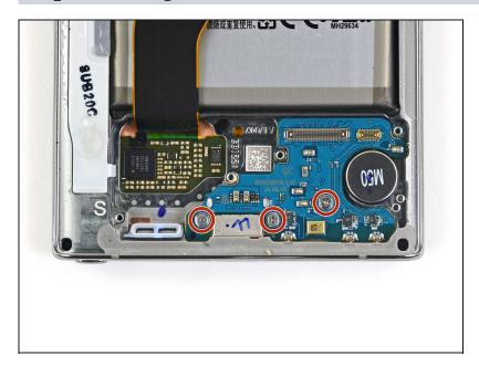
Use a Phillips screwdriver to remove the three 4 mm screws securing the charging assembly.
