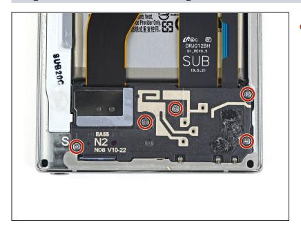
Use a Phillips screwdriver to remove the five 4 mm screws securing the loudspeaker.
