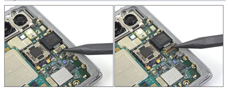
• Use the pointed end of a spudger to pry the front-facing camera connector straight up from the motherboard.
