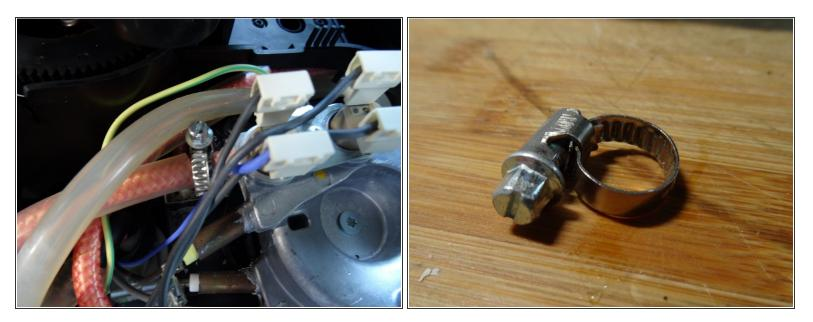
• When reassembling, the Oetiker clamps can be replaced with a 9mm hose clamp.
