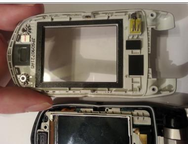
Use a plastic opening tool to remove the screen cover from the rest of the lid.
