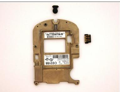
To remove the battery connector simply slide it out from the metal bracket using your hand.
