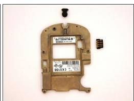
Remove the small black rubber microphone by sliding it off of the metal bracket.
