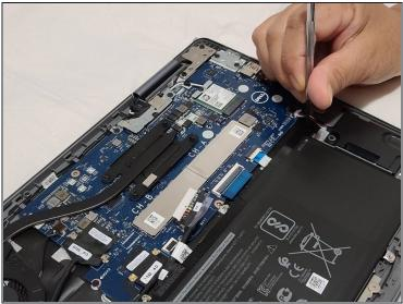
• Using a Phillips #0 screwdriver, remove the four 3 mm screws that secure the battery to the motherboard.
