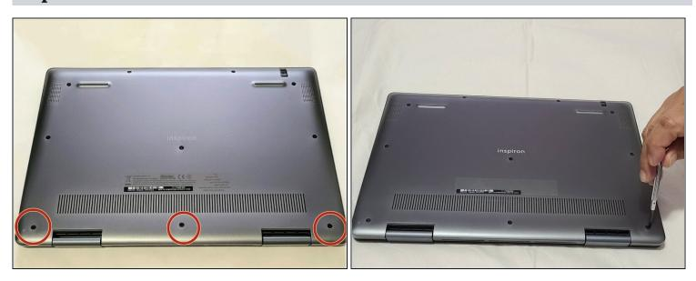
Unscrew the three captive screws with a Phillips #1 screwdriver.
