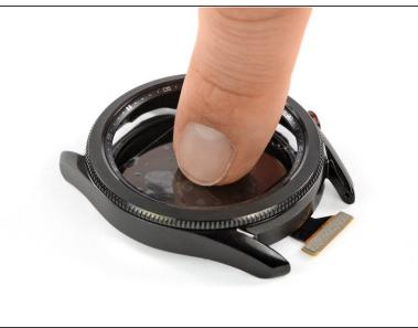
↑ If your display is cracked, keep glass shards contained by applying a strip of tape over the glass."
