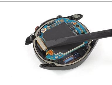
Use the flat end of a spudger to pry up and disconnect the display flex cable from the motherboard.
