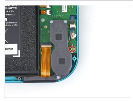
Use a JIS 000 driver or an official iFixit PH 000 driver to remove the 4.5 mm screw securing the left speaker module.
