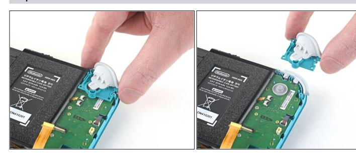
Remove the left trigger button assembly.
