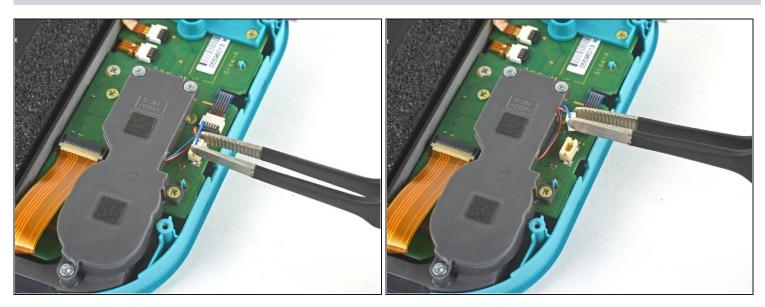
Use a pair of tweezers or your fingers to pull the left speaker cable straight up and out of its socket on the daughterboard.
