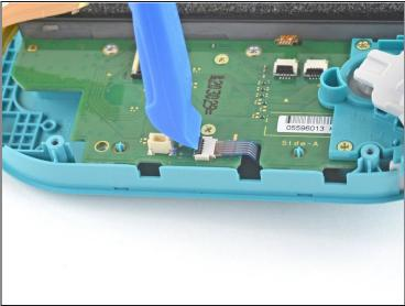
Use an opening tool or your fingernail to flip up the small, hinged locking flap on the left joystick cable's ZIF connector.
