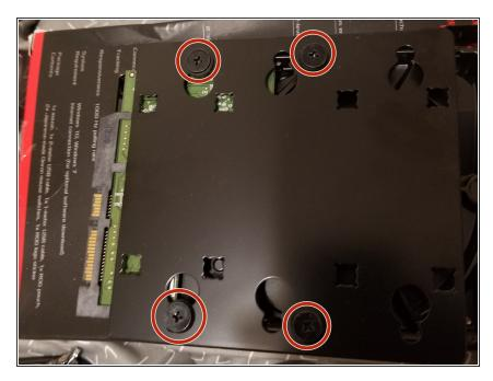
Remove four #2 Phillips screws from the hard drive case in a cross pattern.
