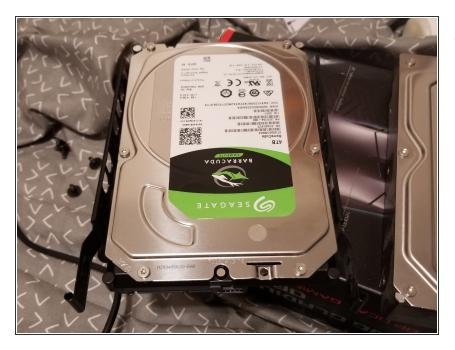
Replace the old hard drive with the new hard drive.
