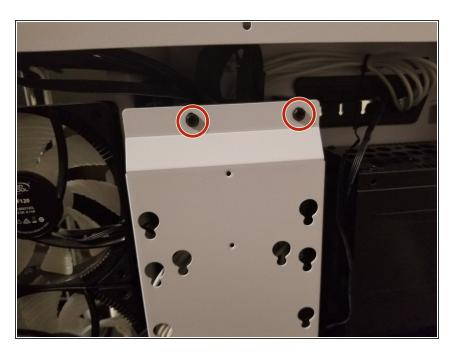
Remove the two 3 mm Phillips #2 screws from the wire cover.
