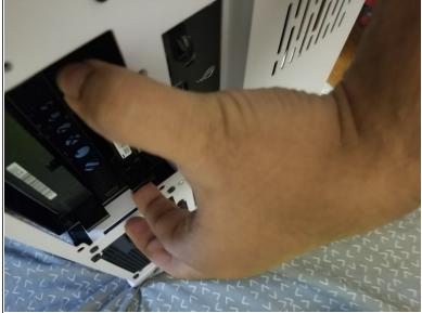
• Push together the bottom and top tabs and pull the hard drive tray out of the case.
