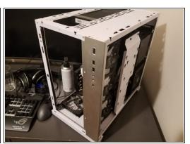
• Remove the remainder of the panels by pulling upwards on them.
