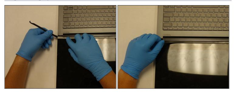
Using a halberd spudger, gently lift up the metal bezel that lines the lower edge of the display.
