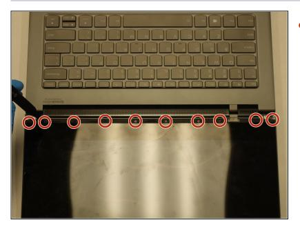
Remove the ten 3 mm screws along the bottom edge of the display with a Phillips #00 screwdriver.
