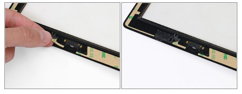
Place the small hook-shaped adhesive strip below the left side of the home button mounting bracket.
