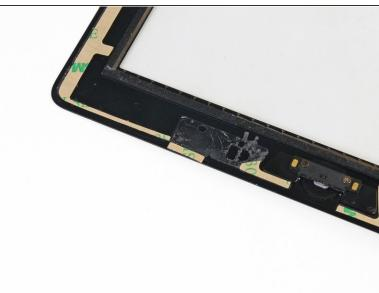
Lay the final small rectangular adhesive strip to the left of the hook-shaped adhesive strip,
