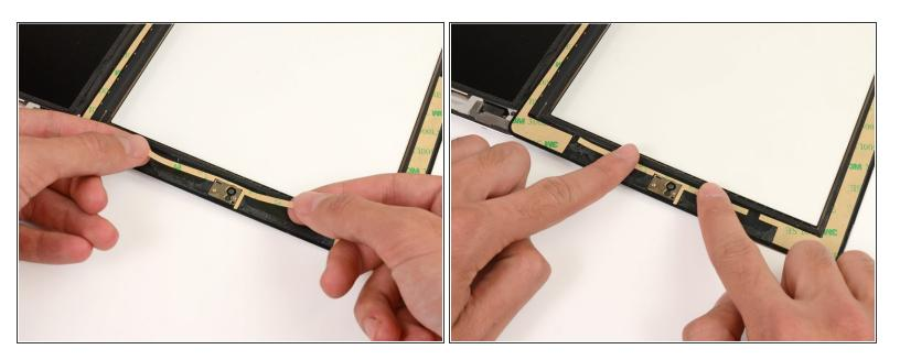
• Lay the thin T-shaped adhesive strip between the bottom edge of the inner frame of the front panel and the camera mounting bracket. The longest edge should be flush with the inner frame.
