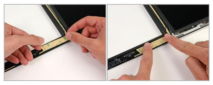
Place the last L-shaped adhesive strip on the bottom right corner of the front panel.
