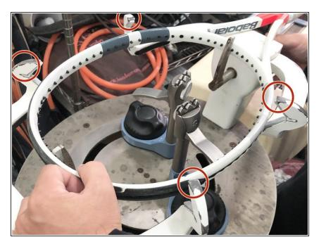
Place the frame into a stringing machine by screwing in the four main screws and pulling the racket tight.
