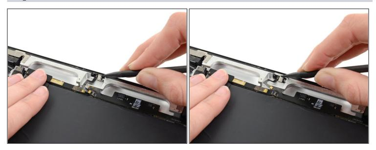
• To loosen the adhesive holding the microphone cable assembly, use a spudger to push it away from the edge of the case.
