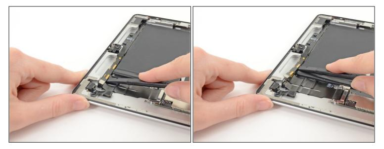
• Use the flat end of a spudger to separate the adhesive securing the front facing camera cable to the control board.
