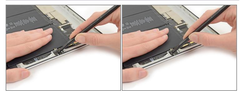
• Using the flat end of a spudger, scrape out any foam adhesive that remains in the front facing camera socket.
