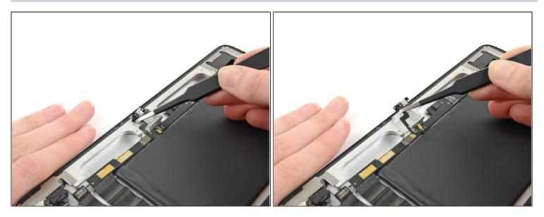
• Remove the microphone cable from the rear case.
