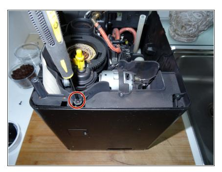
Remove one T10 Torx screw securing the top of the grinder.
