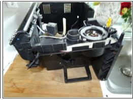
This is what the inner frame looks like from three sides. All components are easily accessible, especially the pump, the flowmeter and the heater.
