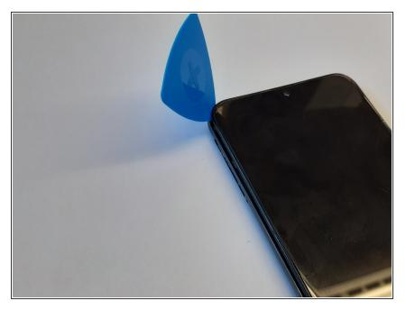
Slide the opening pick along the left edge to the top left corner of the phone, to release the clips.
