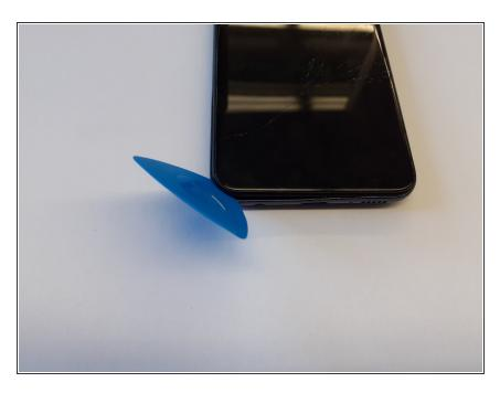
• Slide the opening pick to the bottom left corner to release the clips.
