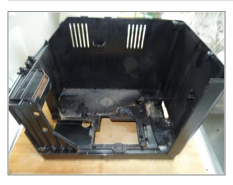
And this is what the completely gutted outer case looks like. It can now be cleaned well.
