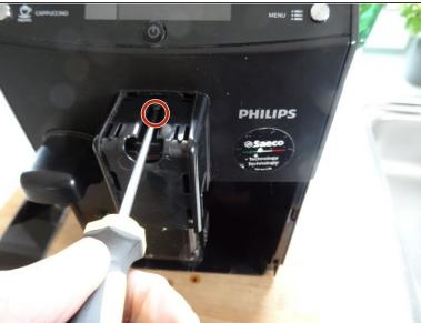
Remove the Torx T10 screw at the top edge of the coffee dispensing spout.
