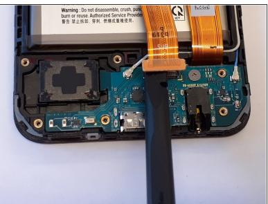
Insert the flat end of a spudger under the interconnect flex connector, and gently pry it straight up.
