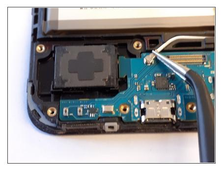
Using a pair of tweezers, gently disconnect the other antenna connector.
