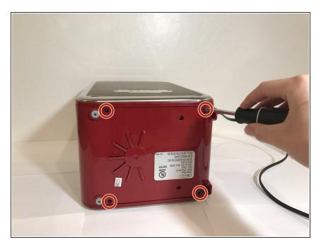
Use a Phillips #1 screwdriver to unscrew the four 3mm screws holding the bottom panel on.
