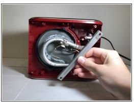
Use a Phillips #1 screwdriver to remove the two 3mm screws holding the curved metal tube in place.
