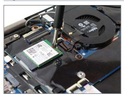
Remove the 2.5 mm screw holding the card in place with a Phillips #1 screwdriver.
