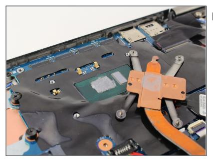
It's best practice to replace the old thermal paste under the 'x' configuration of metal. (Guides on how to replace thermal paste can be found <a href="here">here</a>.)
