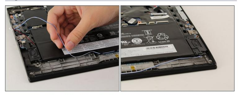
• Unweave the blue and white wires from underneath the plastic tabs connected to the battery.
