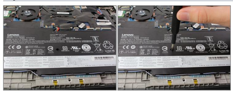
• Remove the central 5 mm screw with a Phillips #1 screwdriver.
