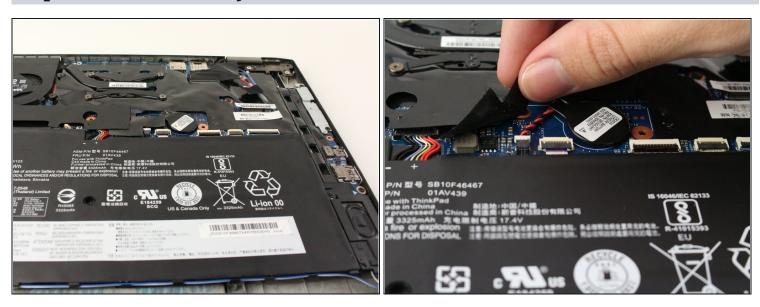
• Peel back the plastic protective cover above the main battery section to expose the coincell's red and black wires.
