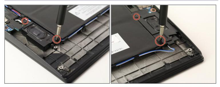
• Remove the two 5 mm screws on each speaker with a Phillips #1 screwdriver.
