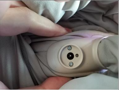
Remove the circular sticker around the charging port. This reveals two screws, which should also be removed.
