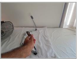
Separate the base from the cage of the fan.
