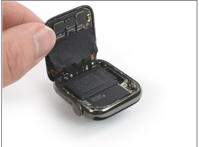
**⚠** Avoid tensioning the display cables when folding the screen to the back.
