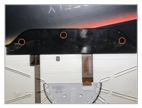
Unscrew the 3 screws with a phillips head screwdriver
