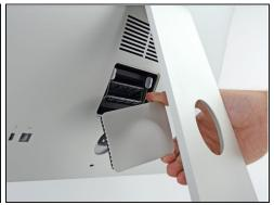
• Pull the RAM access door off the back of the iMac.
