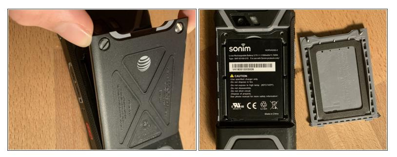
• After unscrewing them, lift up the protective back shield and put it to the side.
