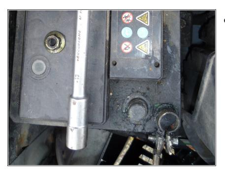
With the 8mm box end wrench, remove the black (ground) cable.
