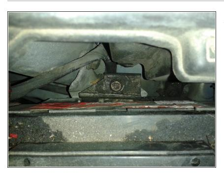
Identify the screw on the right side of the battery which maintains the battery.
