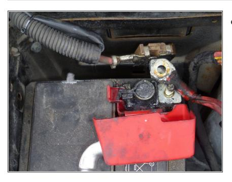
With the 13mm wrench, remove the red cable.
