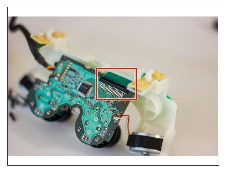
Check the connection of the flexible trigger board to the main circuit board of your controller.
