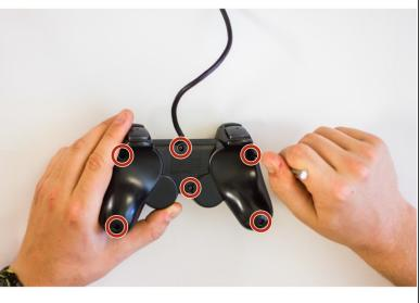
Flip Over Controller and remove all 6 screws from the bottom of the controller.
