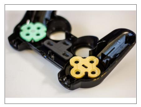
Analyze the rubber pads for any debris that may be getting in the way of the black pads. These make an electrical connection on the pad and may not be contacting properly.
