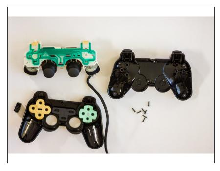
Carefully remove the circuit board from the front cover of the controller.
