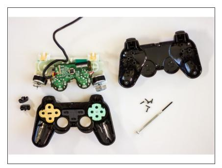
If the previous steps are all covered and you are still facing difficulties in getting your buttons to work, consider replacing the main circuit board or flexible trigger board.
