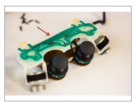
Examine the flexible trigger board itself for any dirt or debris that could get in the rubber button pad's way.
