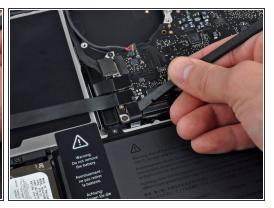
Use the flat end of a spudger to pry the optical drive, hard drive, and trackpad cable connectors up off the logic board.
