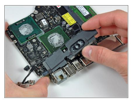
Carefully peel the left speaker/microphone assembly off the adhesive securing it to the logic board.
