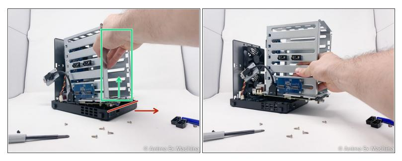
(i) Here, the motherboard is still secure to the disk cage.
