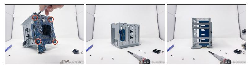
• Once the motherboard is out, unscrew the 4 screws of the metal protective cover (metal plate).
