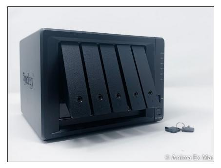
• Before teardown, unlock the disk media with the key.
