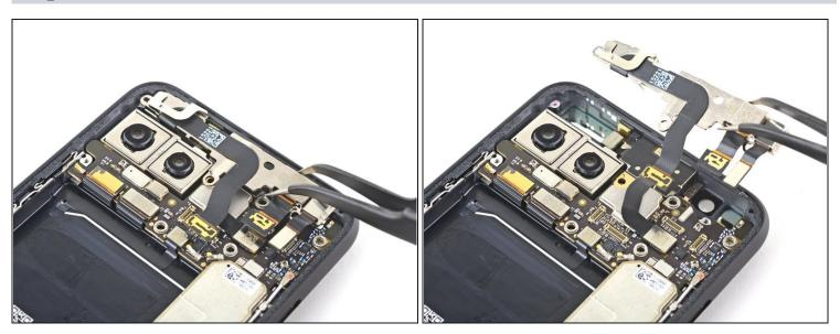
• Use a pair of tweezers to remove the front camera and sensor assembly.
