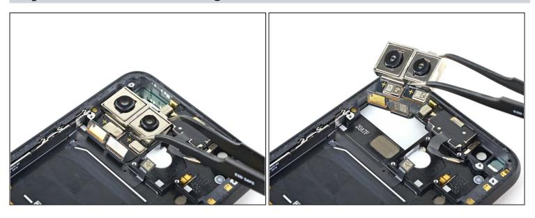
• Use a pair of tweezers to remove the rear-facing camera module.
