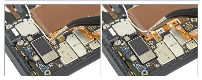
• Use a pair of tweezers to disconnect the antenna connector from the charging assembly by pulling it straight up from the motherboard.
