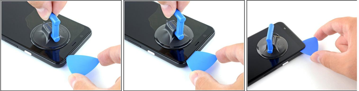
**⚠** This process will almost always destroy the OLED display panel. Only proceed if you are replacing an already-broken display assembly.
