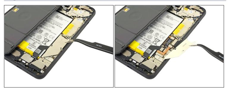
• Use a pair of tweezers to remove the battery connector shield.
