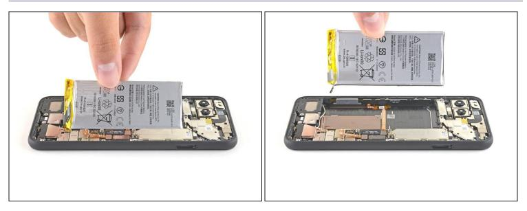
⚠️ Do not reuse the battery if it has been deformed or damaged, as doing so is a potential safety hazard. Replace it with a new battery.
