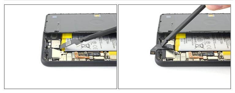
• Using the flat end of a spudger, gently fold the battery cable over so it doesn't accidentally make contact during the rest of your repairs.
