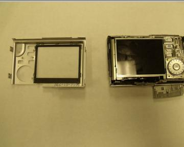
• Separate the back faceplate from the rest of the camera.
