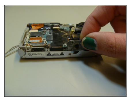
• Remove tripod piece located at the bottom of the camera. This piece should slide out with ease.
