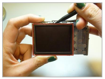
• Use the spudger to pry the LCD from the camera.
