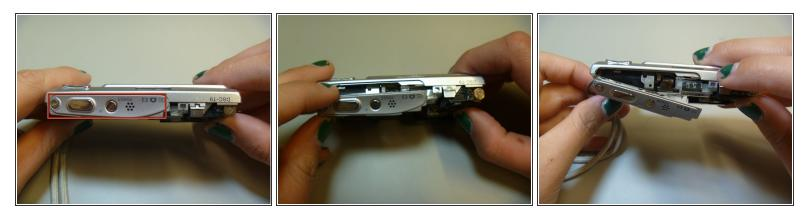
Slide open the top panel. This is located on the top of the camera, where the power button and shutter button are.
