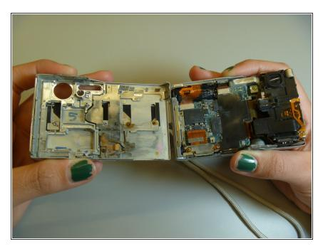
• The front cover is now removed from the camera and the internal hardware is now exposed.
