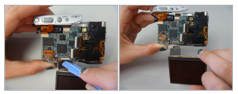
• Use pry stick to pop out LCD connector ribbon, also called the ZIF connector.
