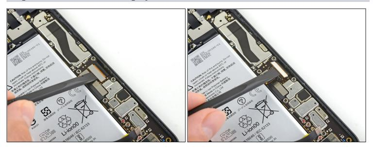
• Use the flat end of a spudger to disconnect the display connector from the motherboard.
