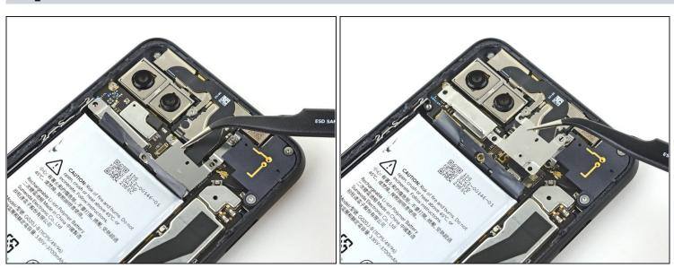
• Use a pair of <u>tweezers</u> to remove the rear-facing camera connector cover.
