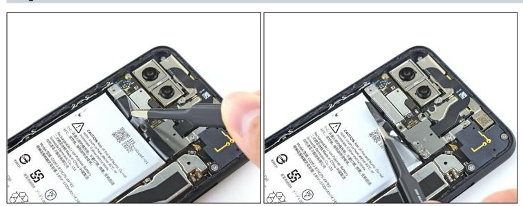
• Gently pry back the battery adhesive pull tab to allow easier access to the screws underneath it.
