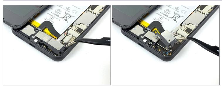
• Use a pair of <u>tweezers</u> to remove the battery connector shield.
