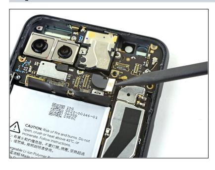
Disconnect the earpiece speaker connector from the motherboard.
