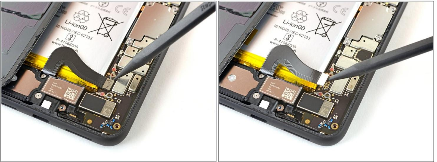
**⚠** Whenever you use the spudger near the battery, be very careful not to puncture the battery.
