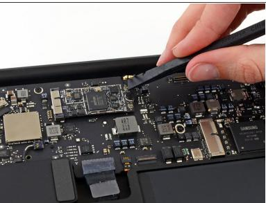
Use the flat end of a spudger to pry both antenna connectors up from their sockets on the AirPort/Bluetooth card.
