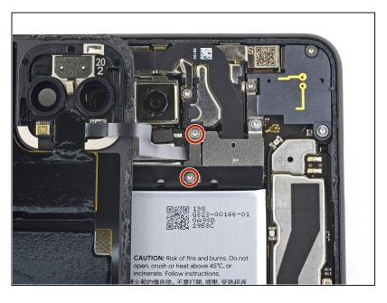
Use a T3 Torx driver to remove the two 4.1 mm screws securing the back panel connector cover.
