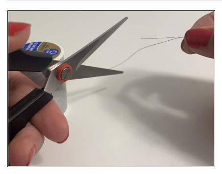
Cut the ends of the thread.
