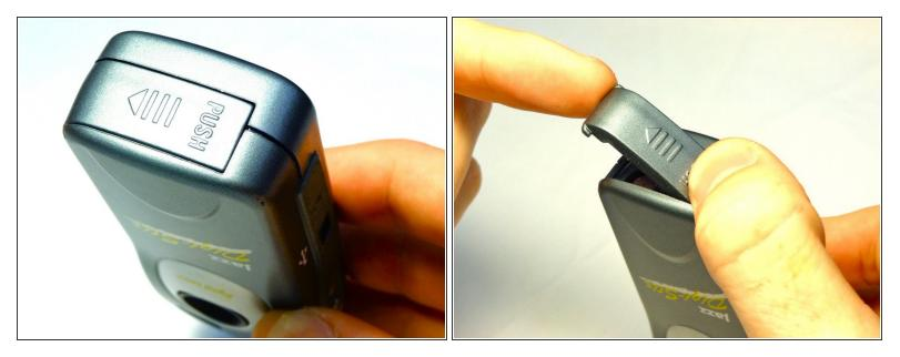
• Flip the device so that the bottom is facing upwards. Using thumb, push the tab on the bottom in the direction indicated by the arrow and then lift the unhinged part of the tab.
