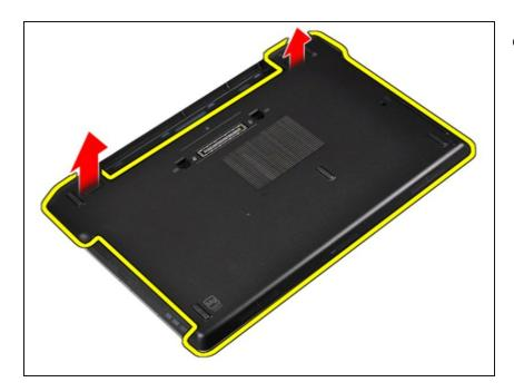
• Lift the base cover to remove it from the computer.
