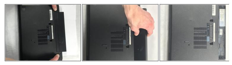
• Slide latches out to unlock and remove battery.
