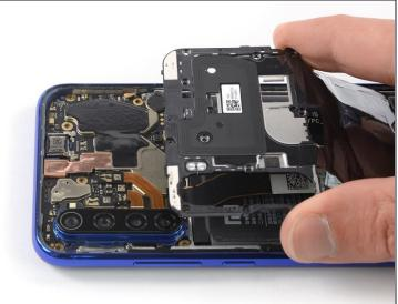
Remove the motherboard cover including the black protective foil that covers the battery.
