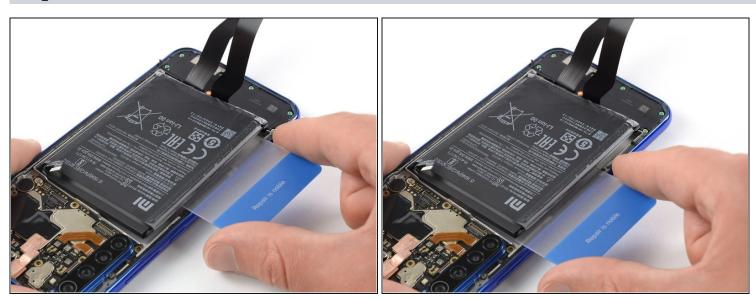
• Slide the <u>plastic card</u> underneath the battery and cut the adhesive with it. Work your way along the left edge of the battery until you've loosened all adhesive.
