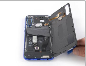
• Carefully fold the rear glass to the right side of the phone. Use the suction handle as a stand for the rear glass.
