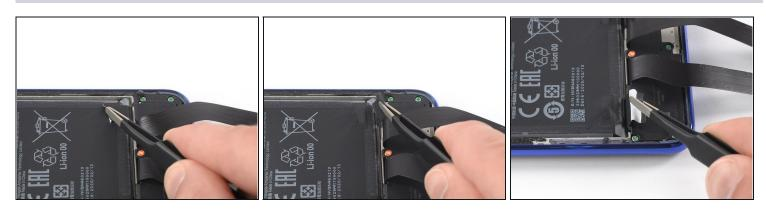
• Use a pair of tweezers to carefully peel the black ends of the two adhesive strips off the bottom edge of the battery.
