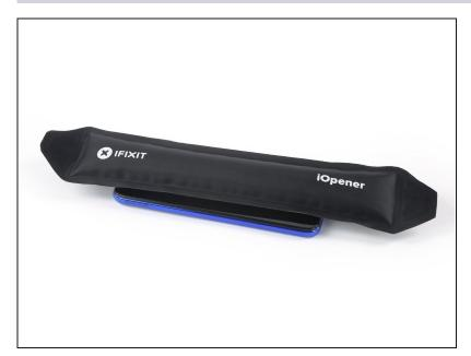
Apply a <u>heated iOpener</u> to the screen to loosen the adhesive beneath the battery. Apply the iOpener for at least two minutes.
